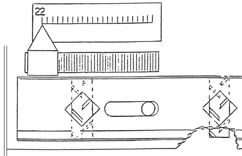
When seeding the grasses listed on page 34, move the feed wheel as shown above. Set the pointer on number 22, the center of the feed wheel should be centered in the opening as viewed from outside of the box. Generally, a small screwdriver or similar tool may be inserted through the opening into the tank and used to push the wheel into position. The agitator blades inside the drill box may need to be re-centered over the feed wheels to prevent interference.
